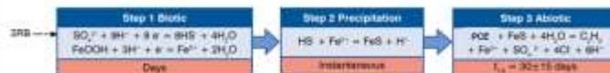
Figure 2: Biogeochemical reduction of chlorinated solvents. SRB reduce sulfate (SO 4 2- ) to hydrogen sulfide anion (HS - ) which reacts with Fe 3+ producing ferrous sulfide (FeS). FeS reacts with chlorinated compounds including PCE, TCE and carbon tetrachloride regenerating SO 4 2- which is reused by SRB to produce HS - allowing the process to continue.
